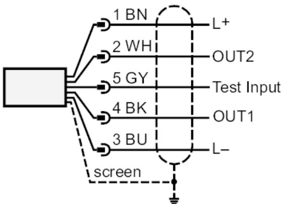
OUT1: Switching output / IO-Link
