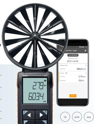
The compact vane anemometer testo 417 was developed to make it as easy as possible for you to take measurements on air inlets and outlets of **air conditioning and ventilation systems**. The integrated 100 mm vane quickly ensures precise results. Time and point average values as well as the volume flow are automatically calculated in the instrument and shown on the display.
